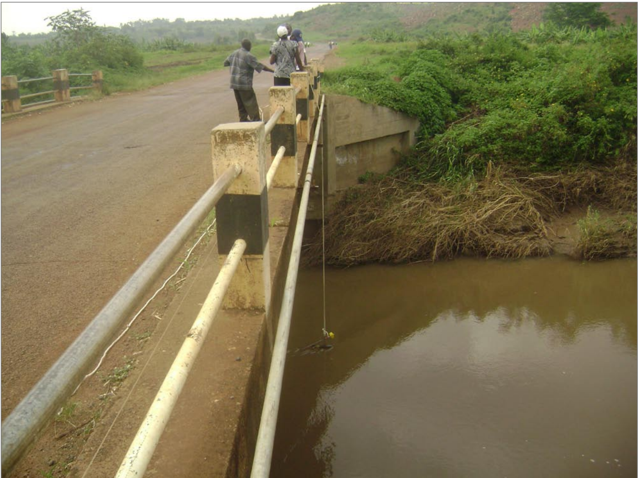
Measuring the discharge at River Manafwa. The silt-covered grass on the river bank shows how high the river rose during peak floods.
